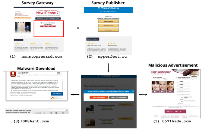
Fig. 2: A case study of online survey scams. The survey gateway (1) asks a set of questions from the victim, and (2) redirects the victim to a survey publisher website. (3) After completing the survey, the victim is exposed to advertisements or malware.
