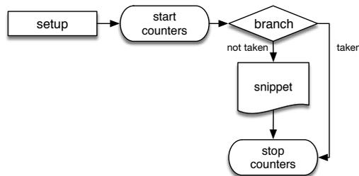
Figure 2: Flow chart of one of the experiment template used in SPECULATOR. The setup code brings the branch predictor in a specific state that will cause the later branch to mispredict and speculatively execute the code snippet consisting of the instructions. The speculative execution of the instructions is measured by the PMC infrastructure, which is triggered by the corresponding start/stop instructions indicated in the flow chart.
