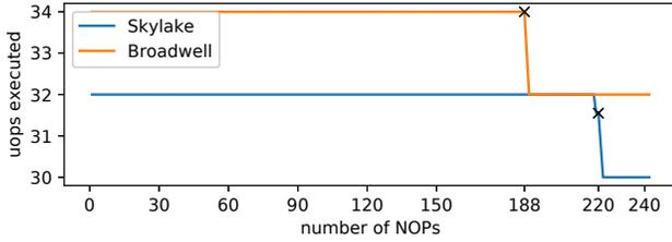
**Figure 7: Reorder buffer size test results on Broadwell and Skylake. Since the marker instruction is no longer executed for a sufficiently large number of NOPs, the number of executed  $\mu$ ops drops at the size of the reorder buffer.**
