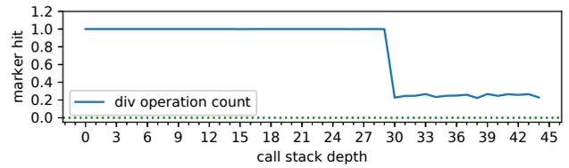
Figure 4: Return Stack Buffer test on AMD Ryzen.
