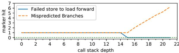
Figure 3: Return Stack Buffer test on Kabylake.
