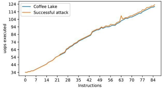
Figure 11: An examination of the SPLIT SPECTRE execution trace between the length check of `string.charCodeAt_at_impl()` and the second array access using SPECULATOR. The graph shows our results of the test on a Coffee Lake machine. It shows that, on average, we are not reaching the second array access in speculative execution. The small spikes in the graph are caused by mispredicted branches in the trace itself, which lead to nested speculative execution of fast-executing code paths.
